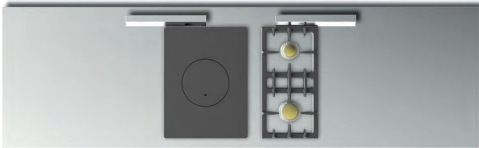
TRADITIONAL HOB 3 BURNERS (5kW BURNER UNDER SIMMER PLATE) 1 burner @ 5kW 1 burner @ 3kW 1 burner @ 1.5kW + 4 integrated hob options
